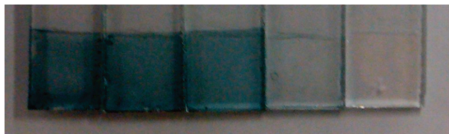
Figure 7. Thin films of PEDOT/PMA containing 0, 16, 80, 90, and 100 wt % Nafion, from left to right, spin-coated and permanently bound to FTO-on-glass electrodes.
